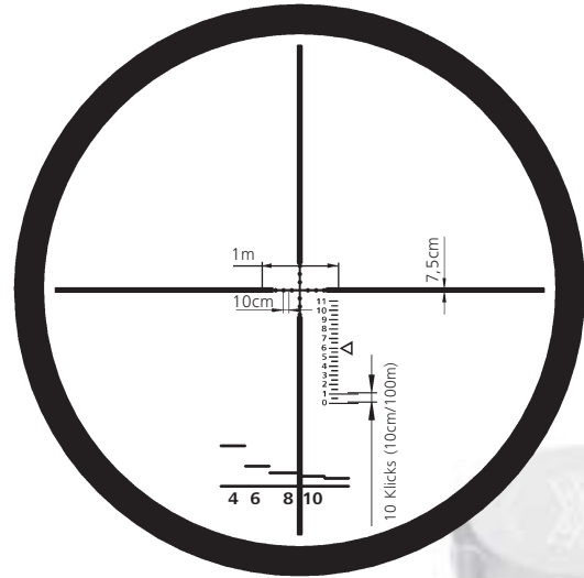
The specified dimensions and MIL DOTS are based on a range of 100 m to the target.
